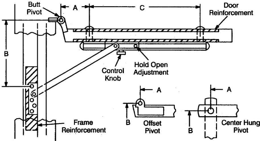
5. Install channel on door with "A" dimension sex bolt. Locate "C" dimension sex bolt hole making sure that channel is horizontal and parallel with stop strip. Drill 1/2" dia. sex bolt hole and finish installing holder. Install control knob on channel as shown.
